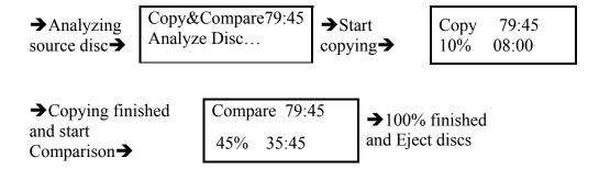
• The Compare Disc function serves as a **bit-by-bit Comparison** between Master Reading Source and the copied discs inside the writer trays. This operation ensures that copies are identical to the Master.
