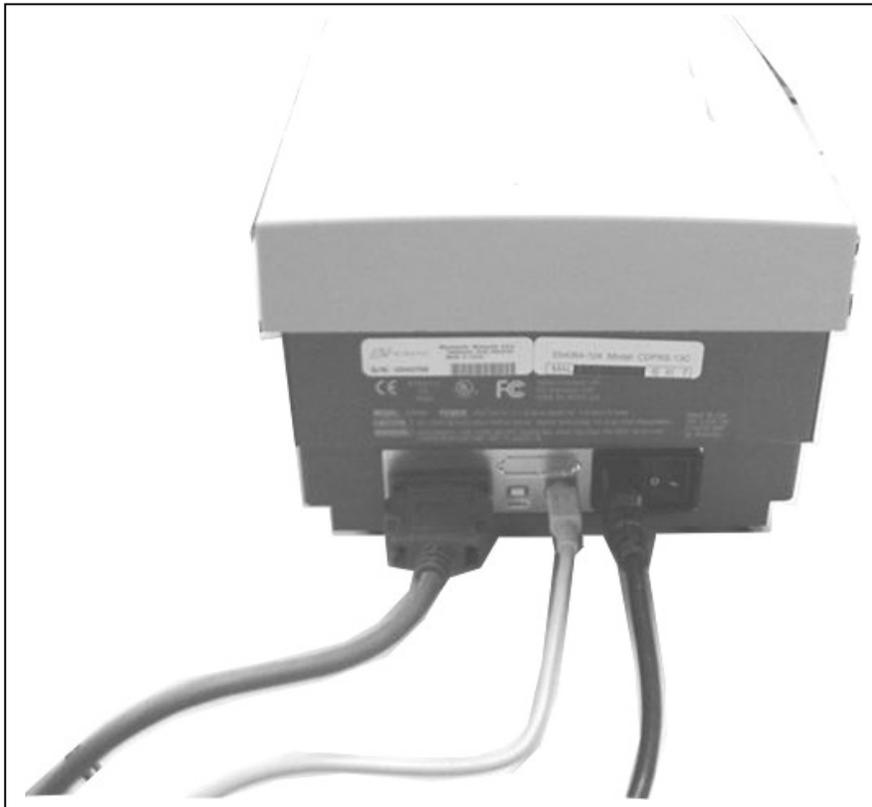
**(fig. 0)** Cabling arrangement for Prism Plus Printer
