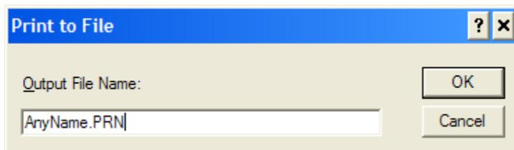
fig. 4 Naming a PRN file. You must use the **“.PRN”** extension to successfully generate a PRN file.
